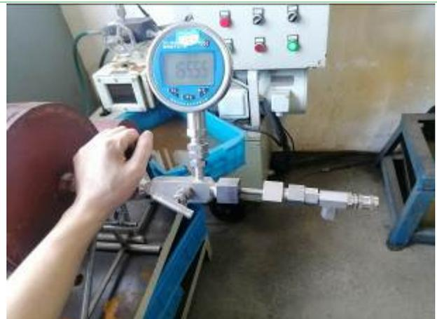
**Fig.32 Pressure test (turn on pressure)**
